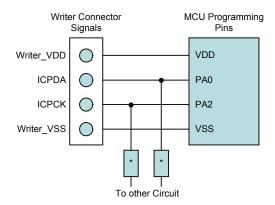
**Note:** \* may be resistor or capacitor. The resistance of \* must be greater than 1k or the capacitance of \* must be less than 1nF.
