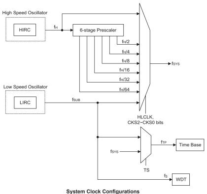
Note: When the system clock source f<sub>SYS</sub> is switched to f<sub>SUB</sub> from f<sub>H</sub>, the high speed oscillation will stop to conserve the power. Thus there is no  $f_{H}\sim f_{H}/64$  for peripheral circuit to use.
