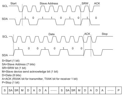
I<sup>2</sup>C Communication Timing Diagram
