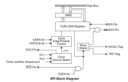
The SPI function in this device offers the following features:
