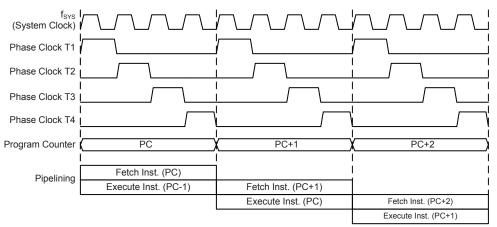
System Clock and Pipelining
