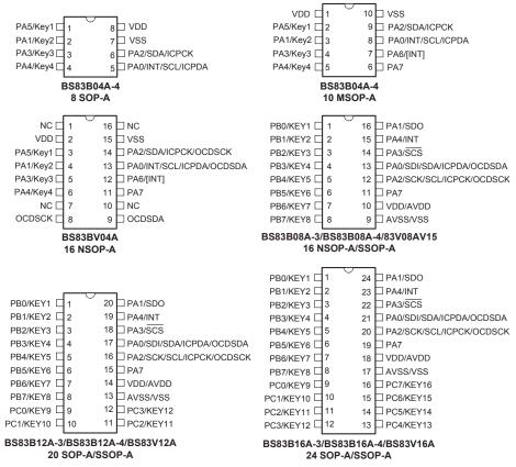
Note: The OCDSDA and OCDSCK pins are used for OCDS function while the ICPDA and ICPCK pins are used for ICP function.
